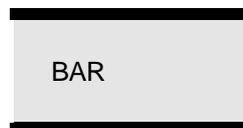
With the [↓] key you can display the process value's unit. Define the unit by selecting **UNITS** from the **CONFIGUR** menu. If user-defined has been selected as linearization function, the text **USER** (default value) is shown as unit.
