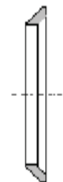
Special adapter for Satron coupling G1 Duplex adapter for installing the sensor head into the coupling (3mm depth)
